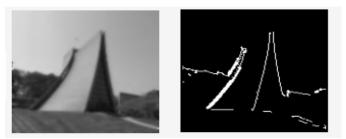
3.Apply Hough transform to find a list of line segments in the image.
